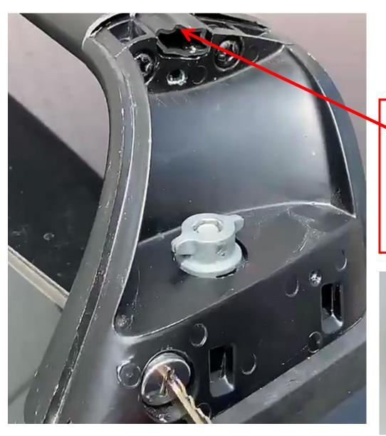
During driving the roof rack will with whistling noise, while even the original Tesla roof rack with this same problem, while please use the wide transparent tape to cover all the rubber grommet. It will helps.
