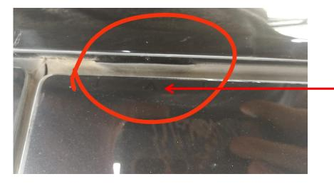
Screw inserted in this position, please make sure the correct positon.
